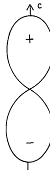
Fig. 4. Polar diagram representing the term \beta_3x_3^3 of V_3 , for all planes containing the c axis.
